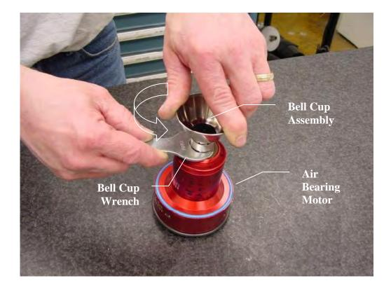
2. Place the cup on a surface that will not damage the cup and carefully remove the cup's insert assembly. The insert assembly may contain more than one piece so exercise caution when removing the bell cup's center components. Use the proper tooling.
