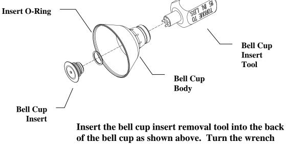
of the bell cup as shown above. Turn the wrench clockwise to loosen the insert from the bell cup body.
