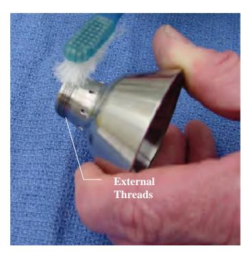
5. Carefully re-assemble the cup with the proper tooling. Care must be taken when reinstalling the bell cup insert assembly into the bell cup body so as not to cut the o-ring on the insert. With a torque wrench attached to the insert tool, insert the bell cup insert tool into the back of the cup and turn the insert counter clockwise (when viewed from the back of the cup). Set the torque wrench to 15 in-lbs. The insert will come to a stop when inserted properly.
